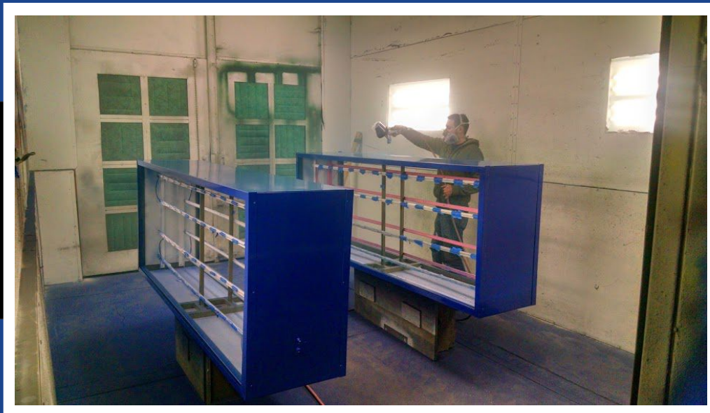
ID cabinets being painted.
