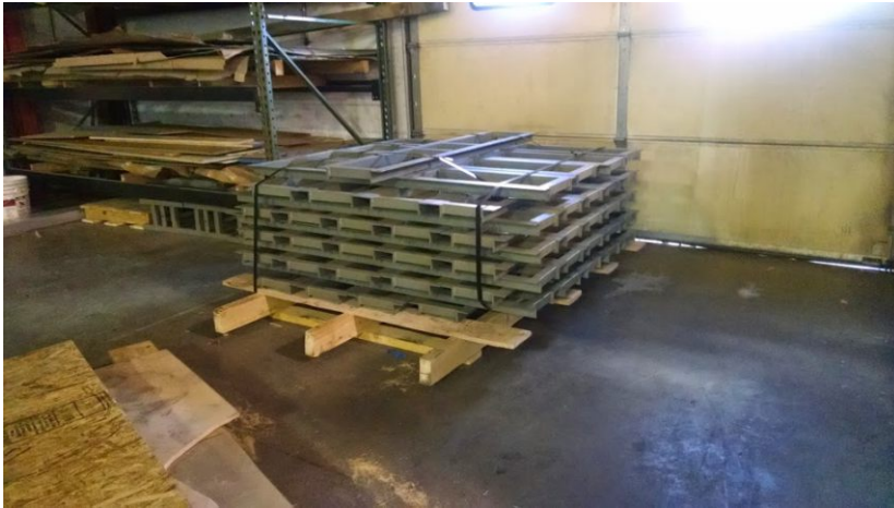
Steel pole cover frames lined up as they were being fabricated. 1" square steel tube
