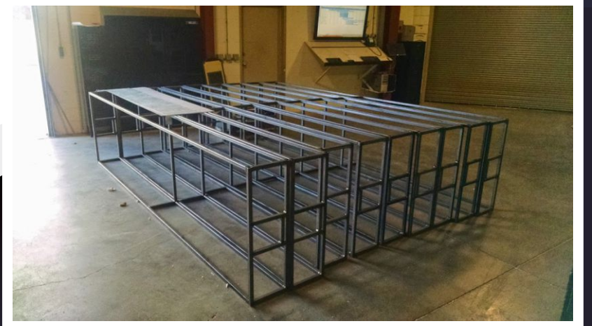
Steel pole cover frames lined up as they were being fabricated. 1" square steel tube
